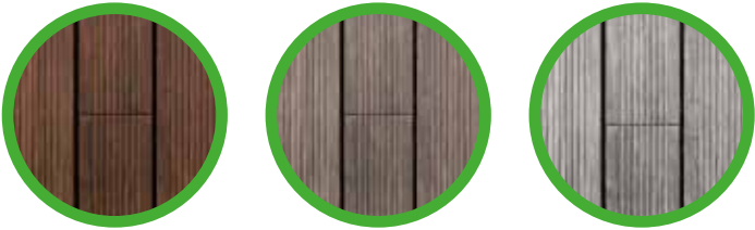
new, non-weathered decking after 3 months of weathering after 18 months of weathering
